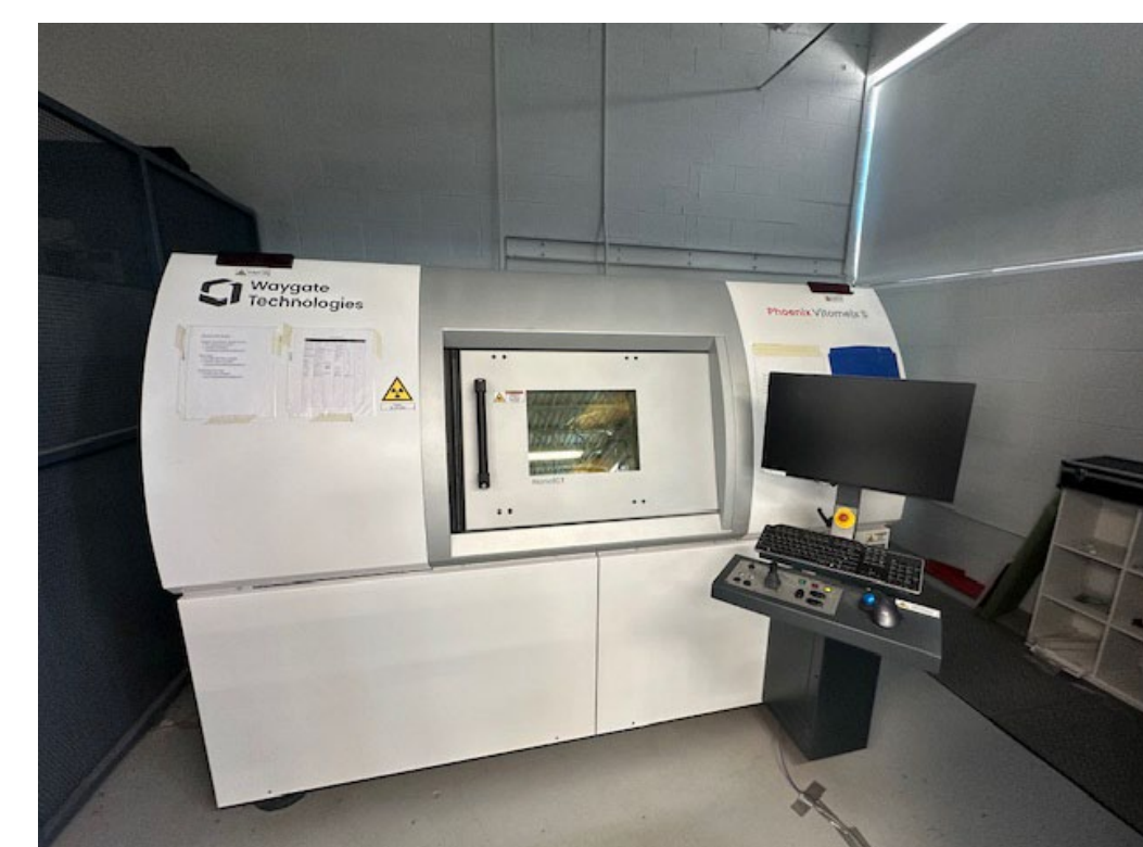
Figure 10. Phoenix V|tome|x S 240 CT Scanning
